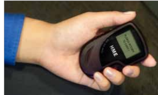
Alphanumeric four-line customizable text messaging. Custom messages can be sent from the convenience of your PC.
